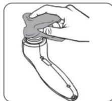
**Clean the device after every use:** With device turned off, clean the ultrasound head probe with a wet towel or soft tissue. **DO NOT** immerse the device in water. Always store device in its protective case at room temperature in a dry location.
