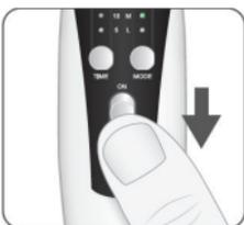
**Turn off the device:** After completing the treatment session, the device will automatically shut off and all indicator lights will be off. Power off the device physically by sliding the power switch downwards (towards “OFF”). Unplug the unit from its power source.
