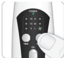
**Set ultrasound intensity:** Press the “MODE” button to select the modulation duty cycle. The mode button has three levels, Low (L) - 5%, Medium (M) - 50%, and High (H) - 100%, each level corresponds to a LED light indicator.
