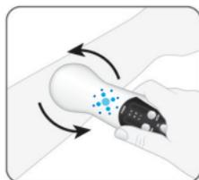
**Place sound head on treatment area and begin treatment:** Move the sound head in a slow, flat, circular motion over the skin surface of the treatment area. Apply the sound head evenly (in time) over the treatment area.
