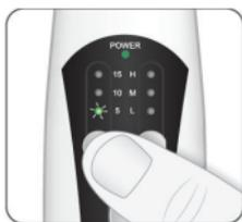
**Set treatment time:** Press the “TIME” button to cycle through the treatment time (5, 10 and 15 minutes), as shown by the “TIME” indicators. When the time is chosen, the system will start working. During working time, the user can press the “TIME” button to adjust the treatment time.
